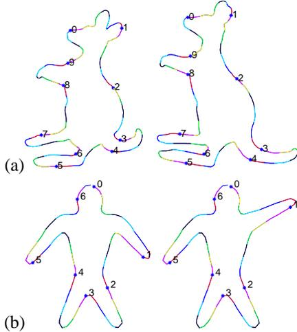
**Fig. 1.** This figure illustrates that the curve matching algorithm works well in presence of view-point variation (a) and articulation and deformation of parts (b). The alignment is indicated by arbitrarily coloring portions of the aligned curves by identical colors with a number indicating the each portion’s end point. Observe that the matches are intuitive, e.g., hands, legs and head of the dolls correspond.
