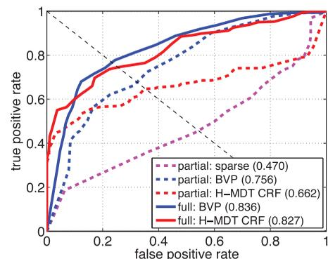
Fig. 8. ROC curves of pixel-level criterion on Ped1.
