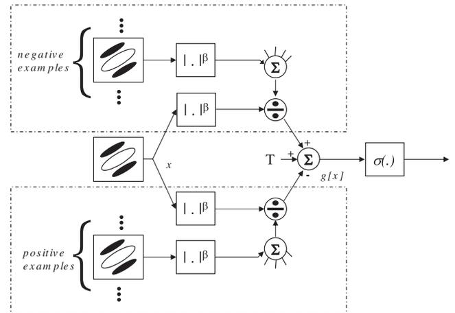
Fig. 7. A LLR unit divisively normalizes a feature response  $x$  differentially, using the outputs of two units that estimate GGD parameters under the target and null hypothesis. With the inclusion of the output non-linearity  $\sigma(\cdot)$ , this unit computes posterior target probabilities.
