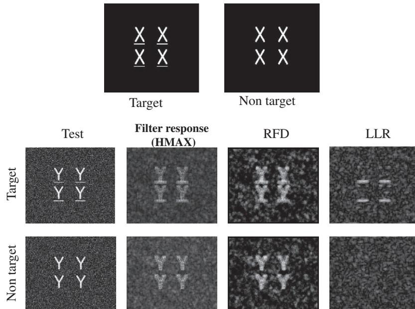
Fig. 9. Detection of underlined characters. Top row: Training examples from target and non-target class. Bottom rows: Examples of test stimuli from the target and non-target class, and layer 1 responses from the three networks considered.
