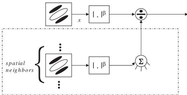
Fig. 6. The NLL is computed by a simple cell that normalizes a feature response  $x$  by the responses of its spatially neighboring units.
