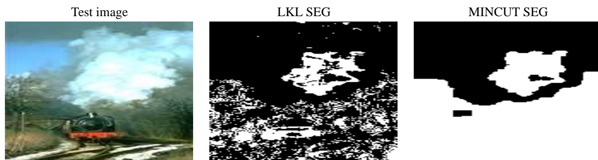
Figure 4. Sky detection results. Dark area represents regions of the image containing the concept sky.
