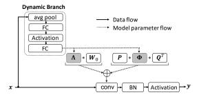
Figure 2: **Dynamic convolution decomposition** layer. The input x first goes through a dynamic branch to generate  $\Lambda(x)$  and  $\Phi(x)$ , and then to generate the convolution matrix W(x) using Eq. 6.
