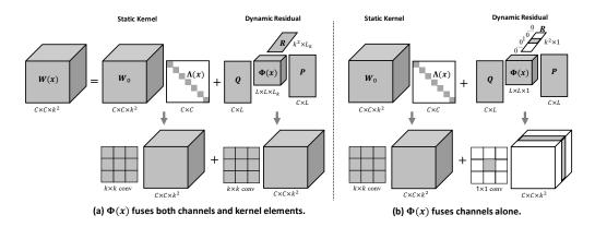
Figure 4: The dynamic convolution decomposition for  $k \times k$  convolution.
