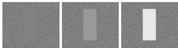
Fig. 4. Bar images with contrast 1.02, 1.07 and 1.78. Background is low variance white Gaussian while bar is uniform intensity.
